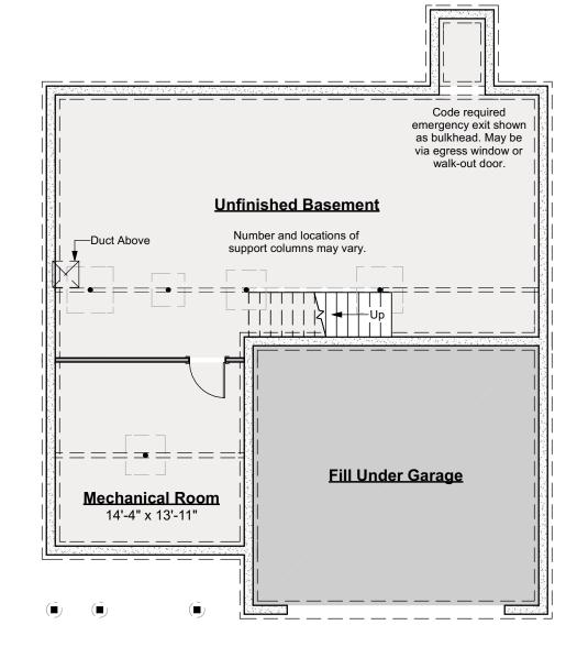
Foundation Plan Scale: 1/8" = 1'-0" CRS 845.124.v16 GR Sir Zach
