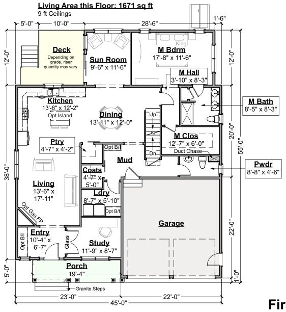
First Floor Plan Scale: 3/32" = 1'-0"
