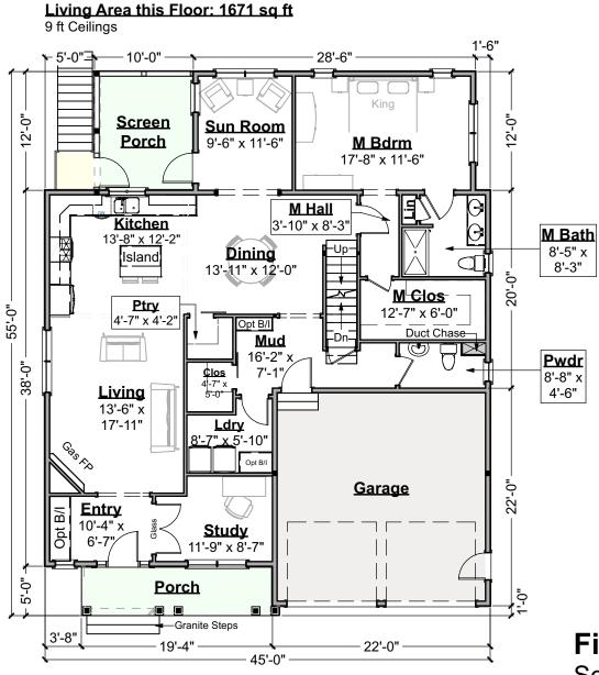
First Floor Plan Scale: 3/32" = 1'-0"
